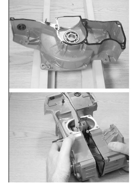
20.19 Place crankcase halves together and align crankcase pins.
